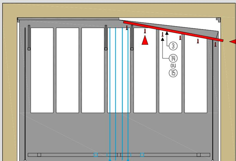
**E** MISE EN PLACE DES PROFILS COTES
