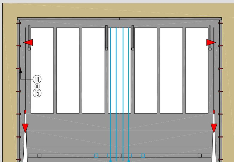
**G** MISE EN PLACE FINALE DES VIS PROFILS COTES
