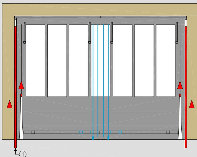
**F** MISE EN PLACE DES VIS SUR PROFILS COTES
